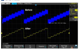
Eres mode can improve the SNR effectively, without the dependence on the periodicity of signal and stable triggering
