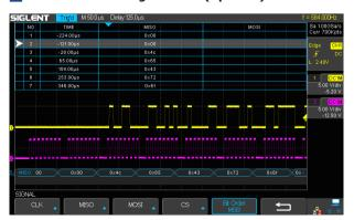
Displays the decoding through the events list. Bus protocol information can be quickly and intuitively displayed in table form
