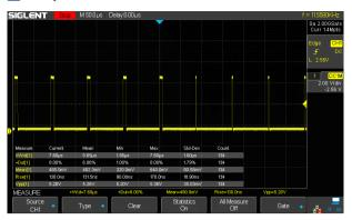
Parametric statistical functions to display 5 parameters of any measurements: current, mean, minimum value, maximum value, and standard deviation. The measurement count is also displayed. The maximum number of measurements that can be run and simultaneously analyzed statistically is five. Supports Gating measurements, Math measurement, History measurement and Ref measurement
