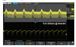
Using hardware-based Zoom technique and record length of up to 140Mpts, users are able to use a higher sampling rate to capture more of the signal, and then quickly zoom in to focus on the area of interest
