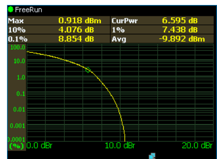
Noise-like signals are analyzed statistically. The average power in this CCDF representation serves as a reference, while the graph shows the distribution of lower power levels.
